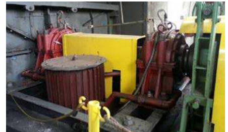
The original sleeve bearings needed all the complexity of continuous lubrication...
