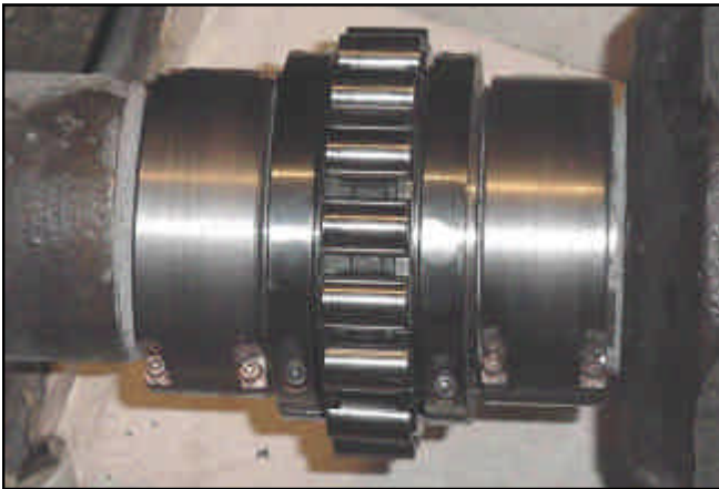
Below: Wear collars shown in position before fitting of housing.
